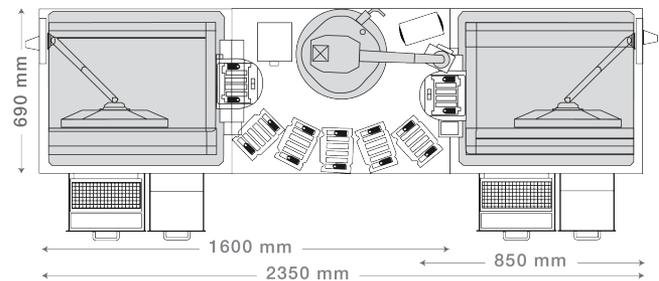
**Figure 2: Dual Scanner AutoLoader 2.x Configuration Example**—Two iScan Systems with an AutoLoader 2.x fit easily on typical lab benches. System height excluding monitor is 510 mm. Additional configurations of the iScan System with AutoLoaders are possible.
