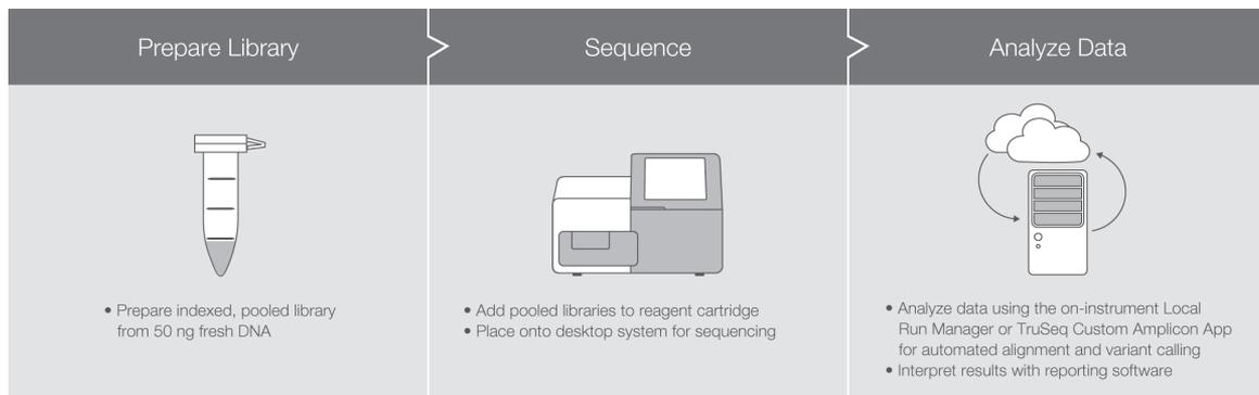
**Figure 1: Simple, integrated workflow**—TruSight Myeloid offers integrated library preparation, sequencing, and automated data analysis, creating a streamlined workflow that can go from DNA to data in three days.
